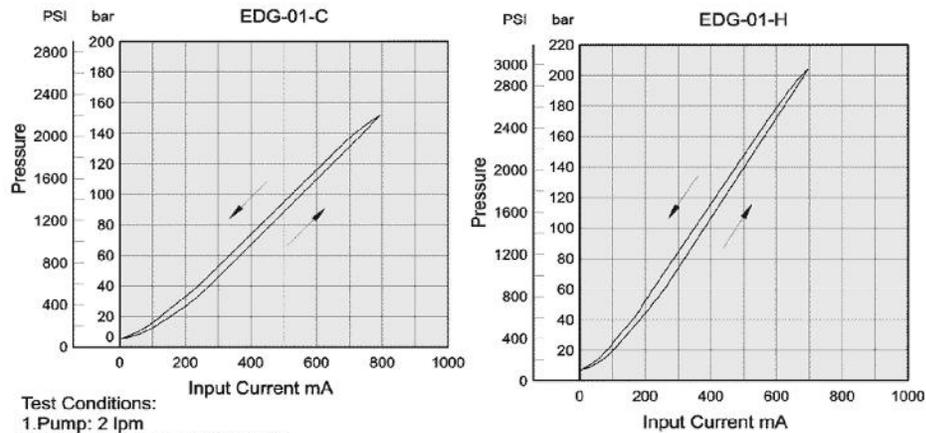
EDG-01 Proportional Electro-Hydraulic Pilot Relief Valves Operating Data
